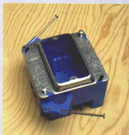
A 4-in. junction box solves most box-fill problems. Throw on a single- or double-gang plaster ring that comes flush with the drywall, and you've got a box that's hard to overfill.
