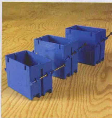
The mere wires, the bigger the box. Single-gang boxes come in three sizes, 18 cu. in., 20.4 cu. in. and 22.5 cu. in. Although smaller is cheaper, larger may avoid box-fill violations.
