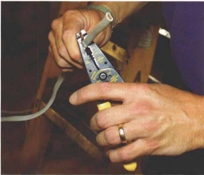
Cable strippers remove the wire's jacket without damaging the conductor insulation.
