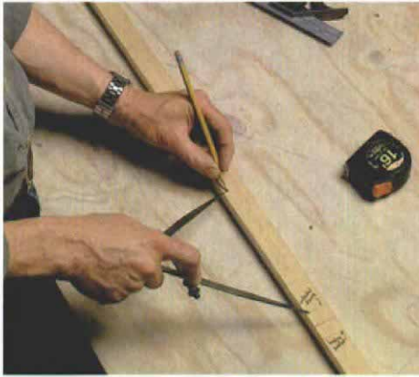
Dividers walk off tread intervals in measured steps. Once he has estimated the rough-tread intervals with a calculator, the author sets a pair of dividers to the interval and makes sure that each tread is equally spaced.
