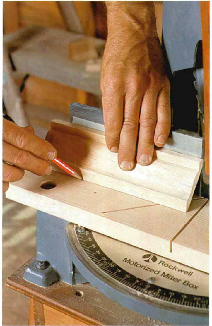
Miter-saw jig keeps correct spring angle. With the gauge block used to mark the crown height on the backing trim, the author transfers a mark to a piece of masking tape applied to the fence (photo top left). This mark corresponds to the mark on the wall measured by the gauge block. Holding a piece of molding upside down against the mark on the fence, the author transfers the molding's angle to the table (photo above). A length of scrap wood keeps the molding's angle proper (photo bottom left).
