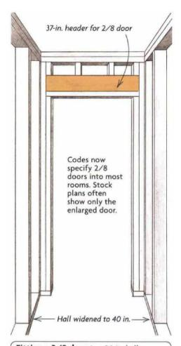
Fitting a 2/8 door in a 36-in. hall requires insetting the kings and jacks in the through walls and ripping the casing. Drywall
