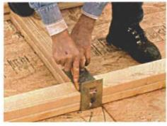
**Channel marker.** This lightweight 31/2-in. wide tool enables carpenters to mark intersecting butt walls on all three sides of through walls with a pencil. A similar tool can be quickly site-built of plate scrap.
