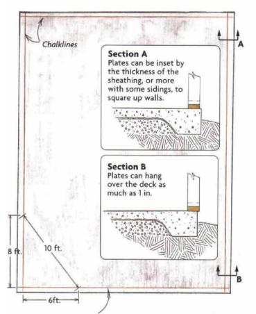
With the long sides parallel, square the perpendicular outside walls. Remember, any triangle whose sides measure 3, 4 and 5, or multiples thereof, is a right triangle.
