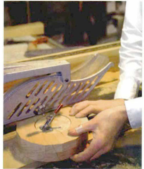
Step 2: Cut the outside circle. A special jig holds the block while the table saw cuts off the corners (left). The blade is then raised slowly while the block is rotated to round the outside edge (right).
