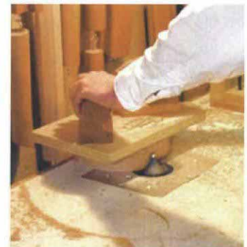
Step 3: Rounding over the outside edges. A jig with a tapered center plug (left) holds the doughnut securely while a roundover bit in a router cuts the profile (right).
