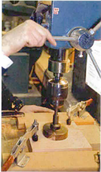
Step 1: Cut the inside hole. After a drill removes some meat in several small holes, a large spur bit in a drill press completes the inside hole.
