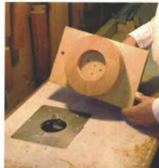
Step 3: Rounding over the outside edges. A jig with a tapered center plug (left) holds the doughnut securely while a roundover bit in a router cuts the profile (right).
