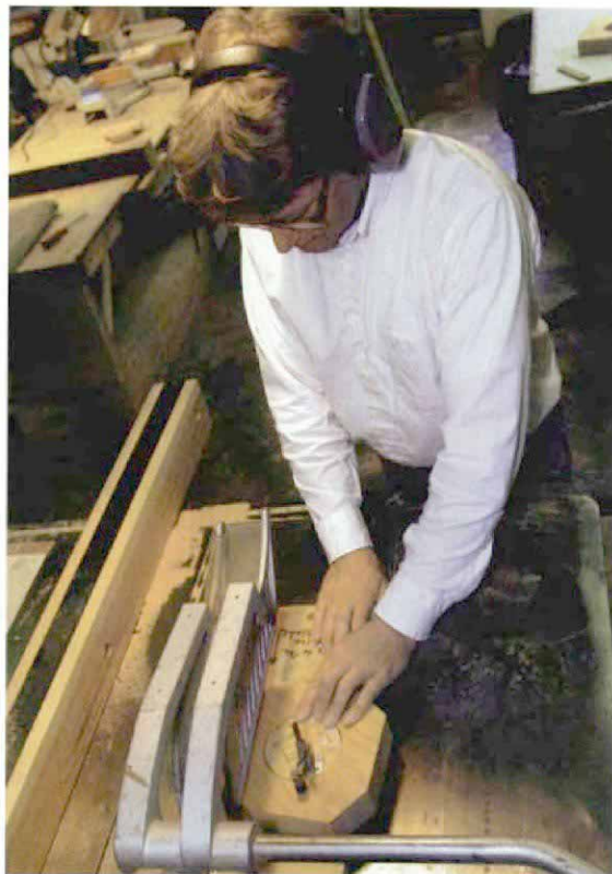
Step 2: Cut the outside circle. A special jig holds the block while the table saw cuts off the corners (left). The blade is then raised slowly while the block is rotated to round the outside edge (right).
