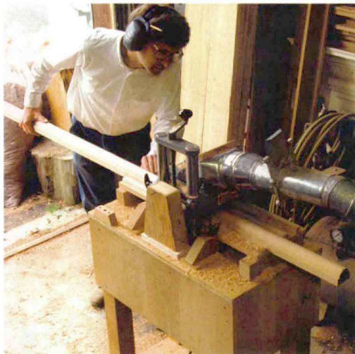
Railing takes shape. Square stock is fed through a molding machine that cuts a half-round profile (photo left). The ledges left on the sides guide the stock while completing the round shape (photo right).
