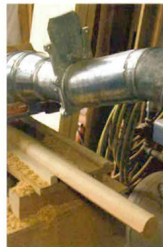
Railing takes shape. Square stock is fed through a molding machine that cuts a half-round profile (photo left). The ledges left on the sides guide the stock while completing the round shape (photo right).
