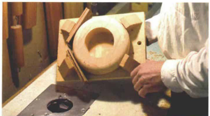
Step 4: Round over the inside edges. Tapered wedges hold the doughnut in a jig that lets the author keep his hands above the work while rounding over the inside edges.
