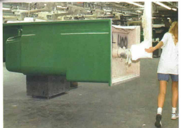
Right this way. A clean polyester-resin mold for a fiberglass-reinforced tub-shower is rolled toward the start of the production line at the Aqua Glass plant outside of Memphis, Tennessee.
