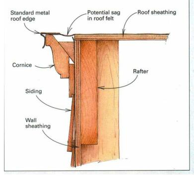
Wide roof edge spans gap. Metal roof edge with a 4½-in. flange will span any gap between a cornice detail and the roof sheathing, preventing sag in roof underlayment and shingles and cutting off a possible source of water leaks.
