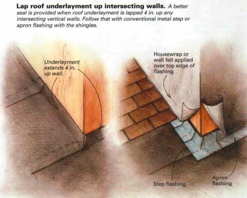
flashing installations, I've found four situations where mistakes commonly occur: around vinyl-clad and aluminum-clad windows manufactured with nailing flanges, at the intersection of a roof and a sidewall (a dormer, for example), where an outside deck intersects the sidewall of a house and, finally, at the edge of a roof. Correctly flashing these spots won't take much more time than doing it wrong, and the effort will save you lots of heartache.
