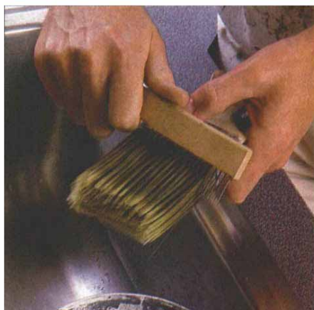
A brush comb straightens out the bristles. When the brush is completely clean, comb the bristles to straighten them out before putting the brush in its wrapper.
