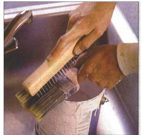
A wire brush removes paint residue. After most of the paint has been washed out of the brush, a wire brushing removes any hardened paint left on the bristles.
