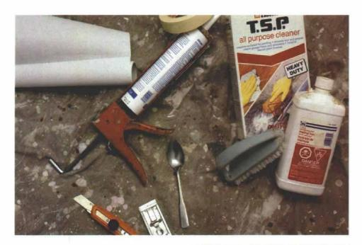
The basic tools are pretty basic. A decent caulking gun—the type with a hexagonal rod and thumb-tab release—a spoon, a utility knife, a scraper, a brush and cleaners are all you need to do a first-rate caulking job. Also bring along plenty of paper towels for cleaning up.
