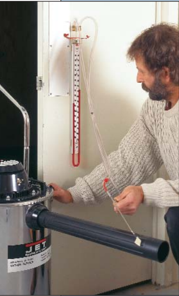
A manometer measures air pressure. A manometer was hooked up in the airstream of each vacuum to measure the suction (negative air pressure) on each machine, which provided common ground to compare the machines.
