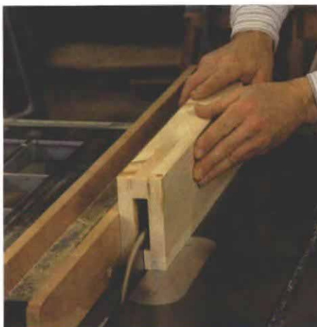
Glued-up plinths are more efficient. To save time and material, the author glues up plinth blocks two at a time, back to back. Then he rips them apart on the table saw after the glue cures.
