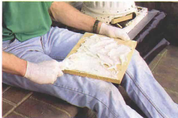
Two-part fillers are mixed on a board. After measuring the right amount of resin and hardener paste, the two are kneaded together on a scrap of plywood.
