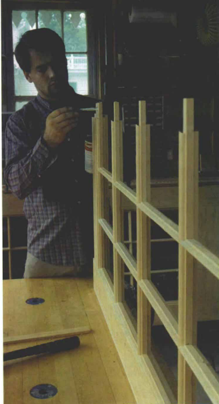
A paintbrush spreads an even coat of glue. After dry-fitting, an exterior-rated wood glue was applied to the mating surfaces of the door, which were then clamped.
