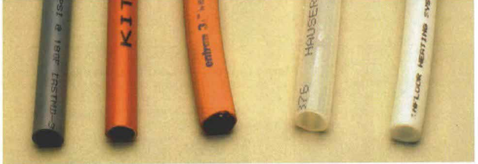
Tubing choices. Left to right: Vanguard polybutylene tubing; IPEX's Kitec PEX-AL-PEX tubing; Heatway's Entran synthetic rubber tubing with oxygen-diffusion barrier; Wirsbo PEX tubing with oxygen-diffusion barrier; and Maxxon's Infloor PEX tubing (without oxygen-diffusion barrier).
