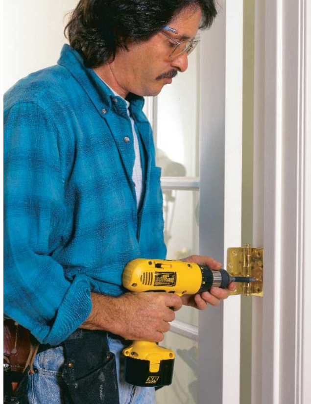
Natural hand position means comfortable work. The weight of the midhandle drill is distributed evenly over the hand so that the hand and wrist stay in natural positions. Pistol-grip drills are nose-heavy and pull the hand and wrist forward.
