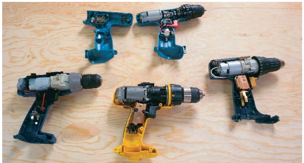
Motor size affects performance. The Ryobi (bottom left) and the Makita (top) have smaller motors that operate less efficiently. The larger motors of the DeWalt and the Bosch (bottom middle and right) are more efficient but weigh a lot more.
