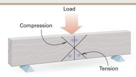
**Extreme fiber stress in bending—Fb.** When a heavy load is applied to a structural member such as a joist, tension is produced in the surface of the opposite side of the board. At the same time, compression is produced in the fibers along the load-bearing surface. Extreme fiber stress in bending (Fb) is a measure of these forces, tension and compression.
