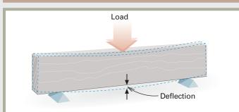
**Modulus of elasticity—E.** Modulus of elasticity is a measure of stiffness. It is a ratio of how much a piece of lumber will deflect, or bend, in proportion to an applied load. E-values provide a conservative prediction of how much deflection might occur in a wall, floor or roof.
