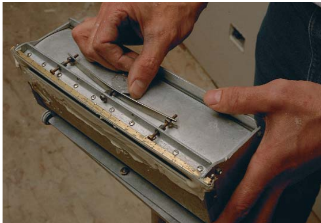
Adjust the blade to control crowning. A dial on this flat finisher sets the curve of the blade, which determines how big the crown will be on the top coat of joint compound.
