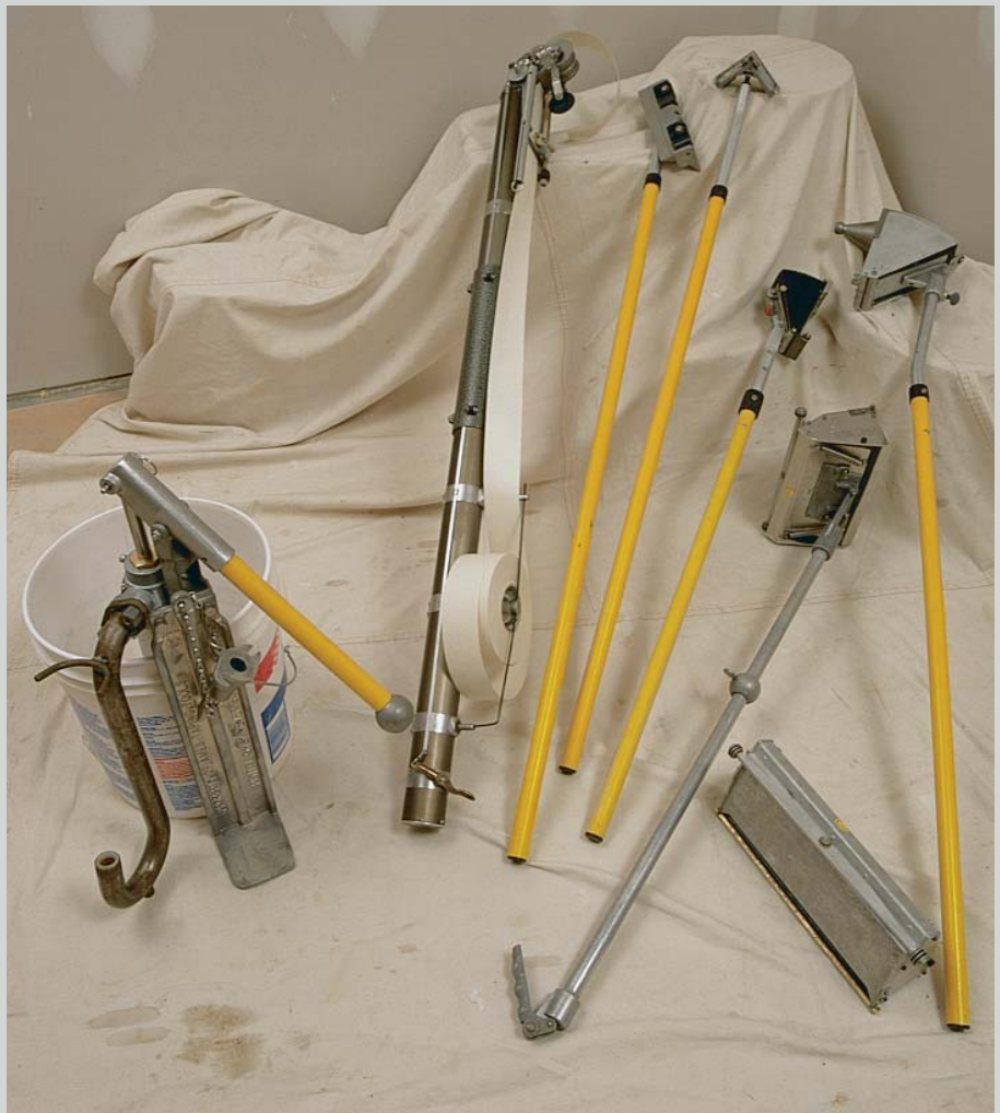
Mechanical tools take you from tape to finish. From left to right, the gooseneck attachment on the Ames loading pump lets you pump joint compound into the Auto Taper, or Bazooka; corner roller; corner finisher; nail spotter; 10-in. finishing box with handle; 12-in. finishing box; and corner applicator.
