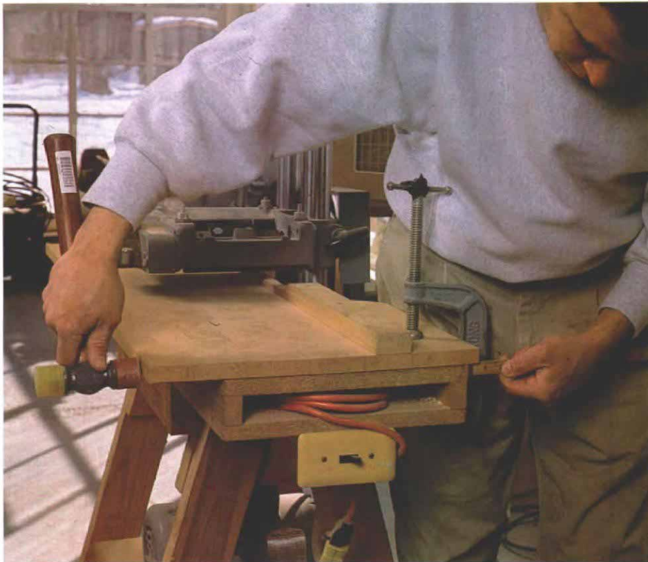
Molder/planer requires a fence. A base-and-fence fixture is clamped to the molder/planer and adjusted so that the fence aligns with the knives. A knife, custom ground with the casing profile, is bolted to the molder/planer's arbor.
