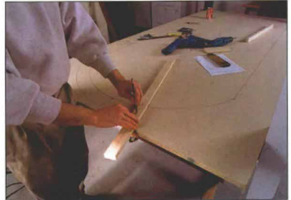
Carved casing from sheet goods. A trammel is screwed to the sheet of MDF and bored so that a pencil can scribe the arched casing.
