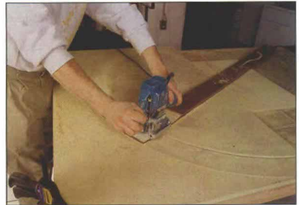
A trammel guides a plunge router. Once the MDF is clamped and screwed to the worktable, the casing's outside radius is cut with a router on a trammel.
