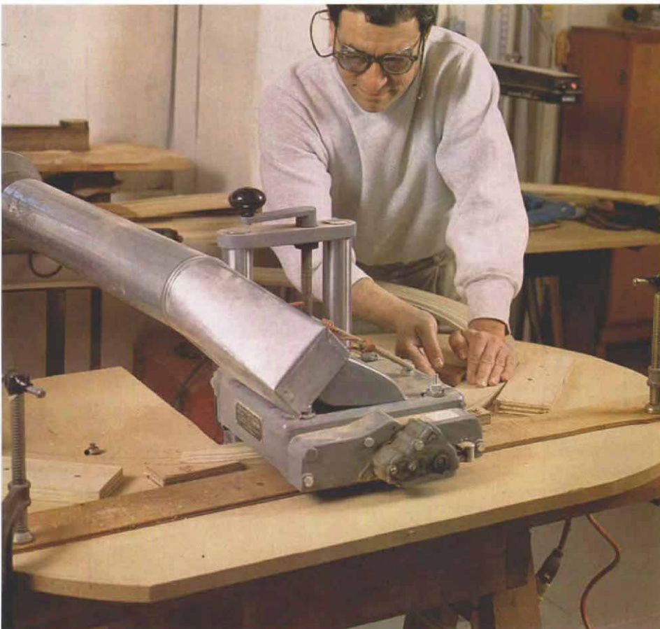
Profiling carved stock. An oversize base, made of MDF, and fitted with a fence and guide blocks, keeps the casing from shifting as it feeds into the molder/planer.
