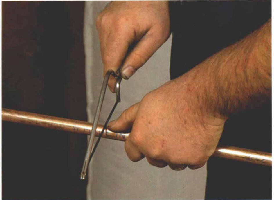
Mark the tubing with a mini-hacksaw. Measurements marked with a hacksaw won't rub off the way pencil and ink do.
