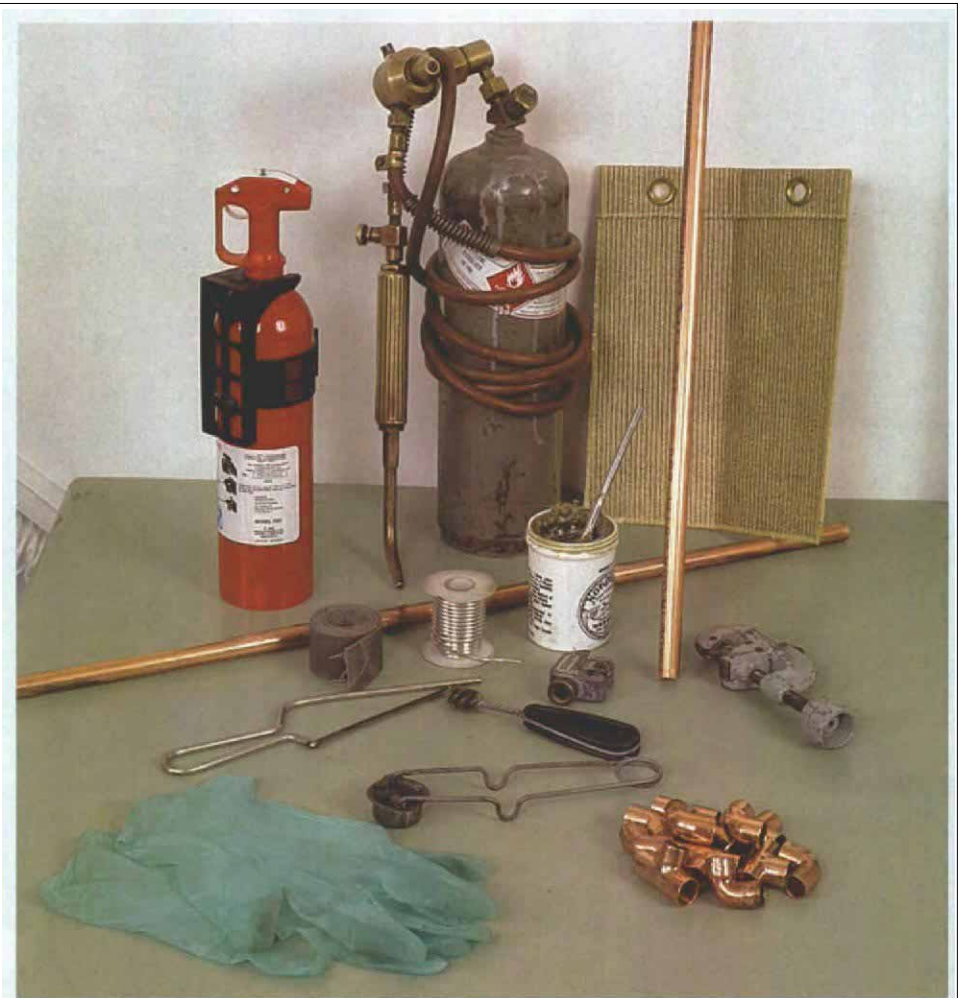
Tools for cutting and soldering copper pipe. This photo shows all the tools needed for basic pipe sweating. Starting in the background: fire extinguisher; acetylene torch with A tank; flame-resistant fabric panel; plumber's sand cloth; lead-free solder; flux; mini-hacksaw; fitting brush; tubing cutter for close quarters; tubing cutter; flint striker for lighting torches; and disposable latex gloves.
