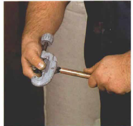
Reaming removes the burr on the inside of the pipe. The triangular blade on the tubing cutter is inserted into the pipe and turned a couple of times to eliminate the sharp edge left from cutting.
