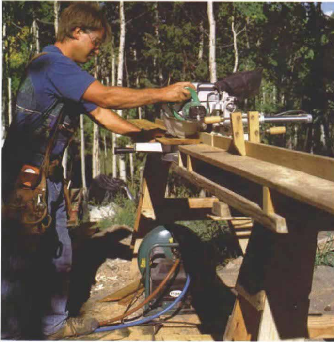
An accurate, portable cutoff rig. A sliding-compound saw, such as the Hitachi C8FB, can make precise crosscuts in siding up to 12 in. wide. Long extension tables support the stock.
