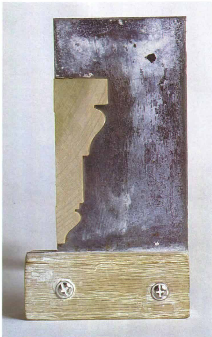
The molding template. The template was shaped to match the molding in the rest of the house. The author added a wooden handle covering the leg to make the tool easier to use and to protect the jamb from being scratched. The trim (left photo) is fashioned of plaster using the template (above).
