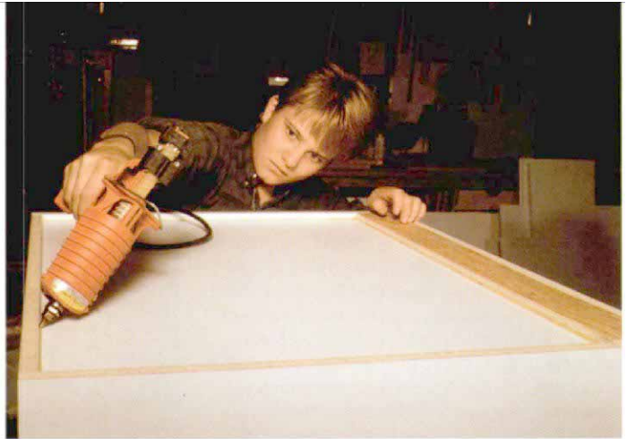
Glue secures the back panel. Karen Umland runs a bead of hot glue around the back panel to affix it to the cabinet's sides, back and bottom. The plywood strip on the right is a hanger bar for the cabinet.
