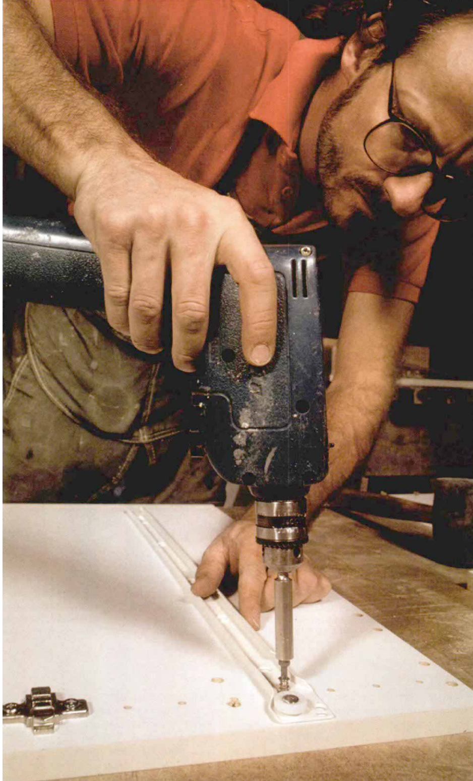
Hardware first. Before assembling the boxes, Michael Fratrack screws the hinges and the drawer tracks to the sides of the cabinet. The holes to the left of the slide receive the doweled drawer divider.
