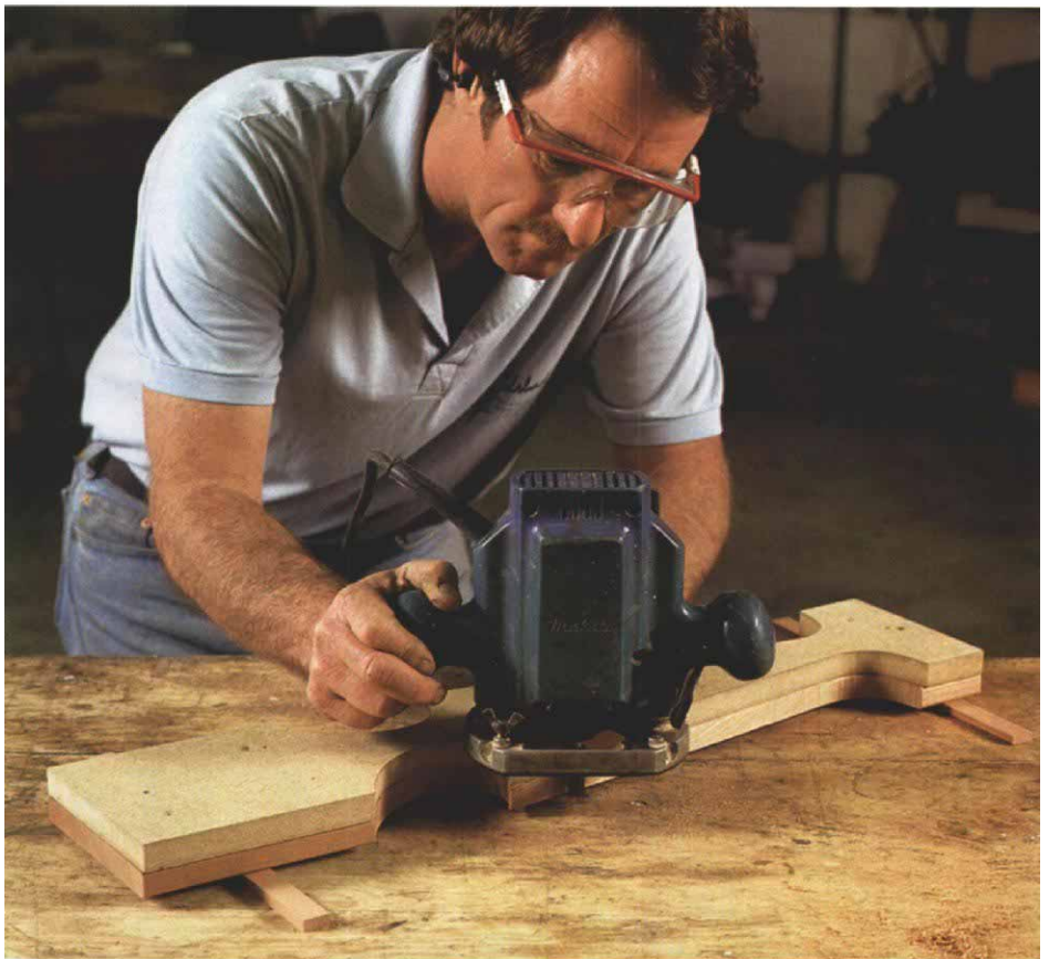
Getting it perfect. Pattern routing involves running a top-bearing flush-trim bit around a template to cut the workpiece. Here, the baluster pattern is tacked to the workpiece below it.
