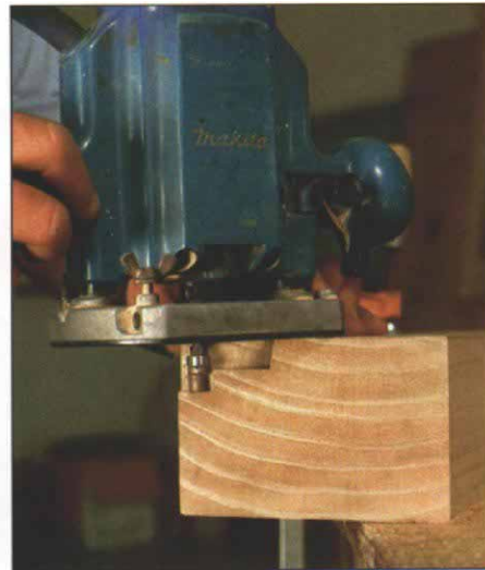
Bit rides against previous pass. Using the same router setup but with the template removed, the author guides the bearing along the cut made by the first pass; in effect, the rafter becomes its own template.
