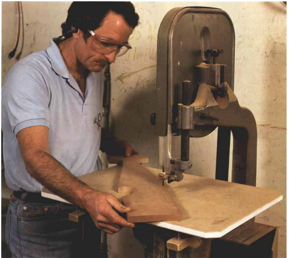
Getting it close. The baluster profile on the 1x6 redwood was sketched from a pattern, then the excess material was removed to within 1/4 in. of the line with a bandsaw.
