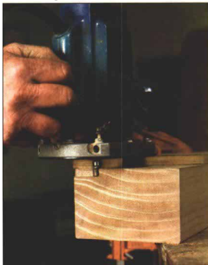
Bit rides against template. With a rafter-tail template clamped to the 4x6 rafter stock, the author guides a ½-in. flush-trim, top-bearing bit along the template's edge to begin shaping the end profile.
