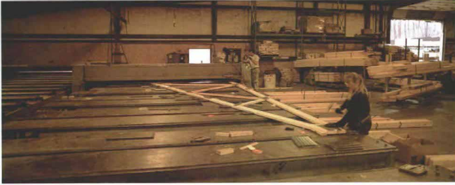
At the factory. Roof trusses are turned out quickly and precisely, thanks to computer-controlled cutoff saws and special assembly tables. At Wood Structures, Inc., in Biddeford, Maine, trusses are assembled either on huge, fixed tables (above) or on movable bases (left). When finished, trusses are moved into the yard on carts that keep trusses upright (below).
