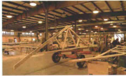
At the factory. Roof trusses are turned out quickly and precisely, thanks to computer-controlled cutoff saws and special assembly tables. At Wood Structures, Inc., in Biddeford, Maine, trusses are assembled either on huge, fixed tables (above) or on movable bases (left). When finished, trusses are moved into the yard on carts that keep trusses upright (below).
