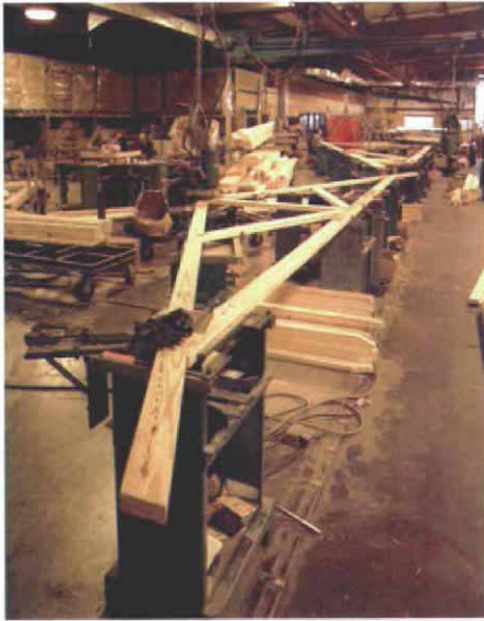
At the factory. Roof trusses are turned out quickly and precisely, thanks to computer-controlled cutoff saws and special assembly tables. At Wood Structures, Inc., in Biddeford, Maine, trusses are assembled either on huge, fixed tables (above) or on movable bases (left). When finished, trusses are moved into the yard on carts that keep trusses upright (below).
