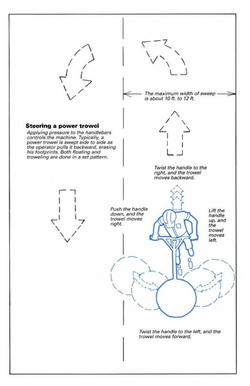
Subsequent passes over the concrete occur with increasing pitch angles ( $10^{\circ}$  to  $20^{\circ}$ ) and depend on how smooth and hard a finish you desire.
