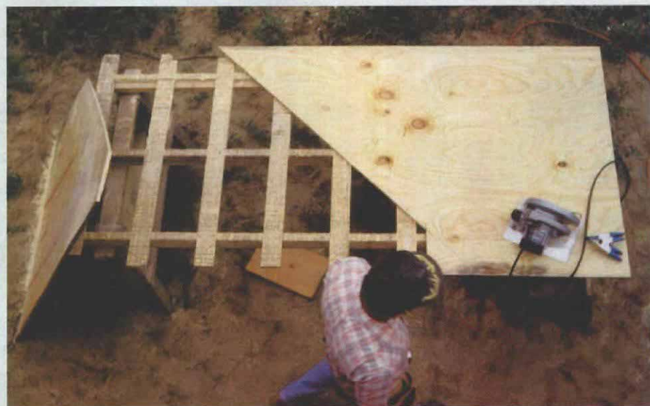
Trouble-free cuts. The grid, supported on a pair of sawhorses and teamed up with a saw guide, helps guarantee accurate cuts on sheets of plywood. Offcuts won't bind the sawblade, and the lack of metal fasteners means you won't damage your blade when making a cut.
