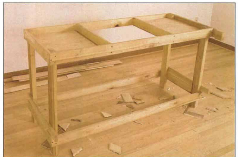
Door bench. This slightly different design also has adjustable cleats to hold a door, but it includes two tool shelves and an open space in the middle of the top where you can stand and walk the bench from room to room.
