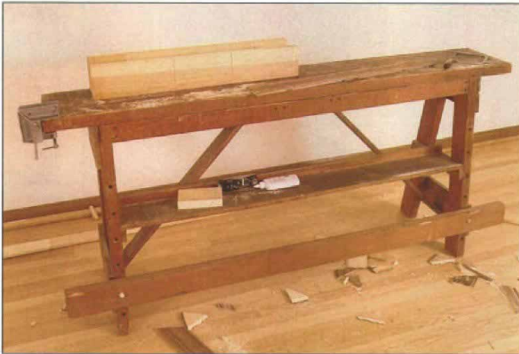
Carpenter's bench. This bench is made from materials commonly available on a job site. The pair of 2x4 legs in the back are slightly splayed to increase stability. An adjustable support on the front will hold a door.
