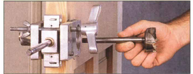
8. Remove the spur bit from the jig before drilling the edgebore.
