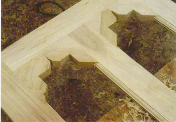
1. Filling the corners. To accommodate the arched, leaded-glass panels in the master-bedroom door, the author glued up four filler blocks, coped them on a shaper and glued the blocks into the panel openings.
