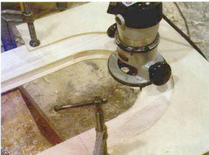
3. Routing recesses. To allow installation of the panels, the author then removed the sticking on one side of the door using a router guided by a second plywood template screwed to the door.
