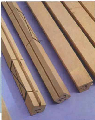
Just a pinch. To keep the staves intact during glue-up, White does not cut the mortises all the way through.
