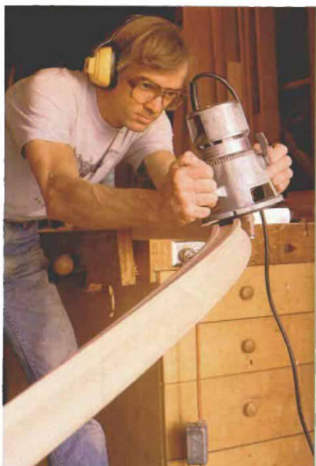
Shaping the handrail. White makes several passes with a custom ogee bit to shape the handrail. The groove in the underside of the rail was cut with a 1-in. straight bit.
