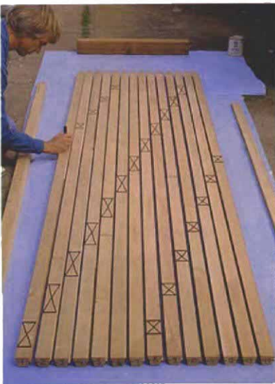
Coopered column. The author marks the entry and exit mortises on the collated staves prior to precutting the mortises.
