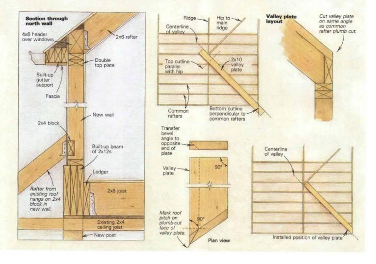
its ridge because of plans to install a heating duct there. There were no horizontal top plates to stop the top of the wall from spreading as we added the weight of the rafters in that bedroom, as well as the rafters supporting the main ridge. When we spotted the problem the wall was out of plumb by ¾ in., and we had the uneasy feeling that the error was compounding at a slow but steady pace. We needed a quick and effective fix.
