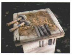
If you are doing a lot of cutting, a banker will make it easier. The one shown above is built from plywood sandwiched between a pair of 2x2 frames and filled with sand on top. The principal tools for working stone on a banker are, left to right, a 3-lb. sledge (two styles are pictured here), a point, a flat chisel, a pitching chisel and a tracer. The cutting tools in the photo have heavy-duty carbide tips.
