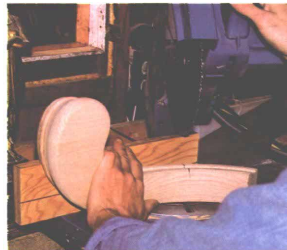
Wherever the shape of the fitting makes it difficult to maneuver in the miter box, the author screws a piece of plywood to the bottom of the fitting as a jig. Here he's cutting a turnout easing with newel cap.
