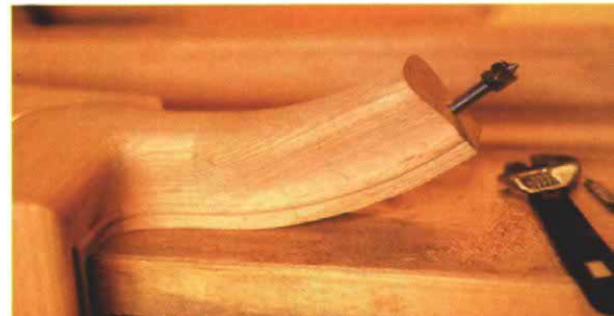
These photos show a gooseneck fitting with a newel cap, quarter turn and an up easing. In the top photo the pitch block is being used (run side down) to locate where to cut the up easing. This procedure is the same as for any starting fitting, since at this point the up easing is the start of a new flight of stairs. In the next photo, the pitch block has been flipped over (rise side down) to mark the angle at which to cut the up easing. The photo above shows the fitting after it has been cut and with a rail bolt attached. The two hex nuts on the rail bolt were locked against each other and used to turn the rail bolt into the up easing.
