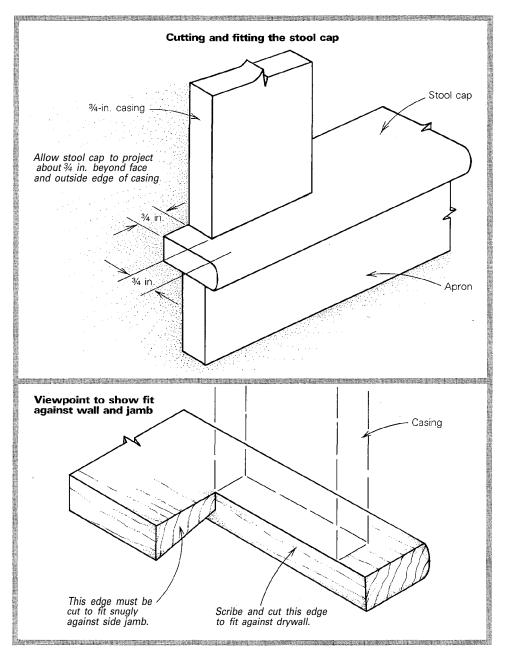
designed so there can be a slight reveal where the casings meet the jambs. Others (like the window shown in the drawings) have a flush fit.
