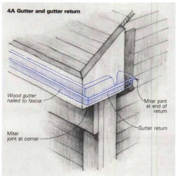
tight, it's a good idea to use a weatherproof adhesive caulk. Phenoseal (made by Gloucester Co., Box 428, Franklin, Mass. 02038) and other marine adhesives work well in this type of joint. I also staple a piece of building paper behind the ear board.
