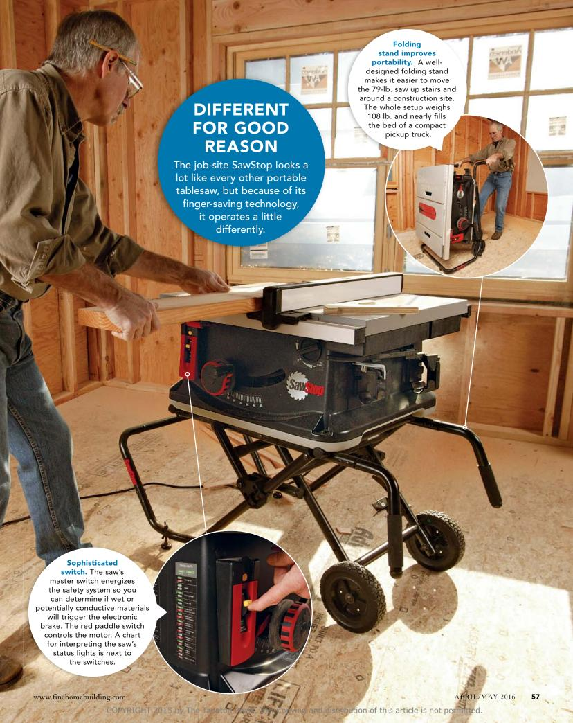
the end. Poke your finger into the toggle to release the fence, slide it where you want, and rock down with the heel of your hand to lock the fence in position.
