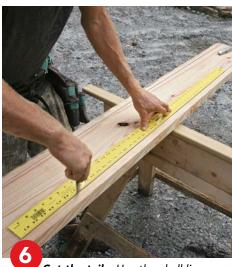
a reference when marking the depth of the notches on the top and bottom of the tail, and connect them with a sharp pencil, which won't wander to follow the grain.
