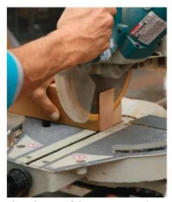
**Slope the tops of the posts.** To give the cap railing a slight pitch while keeping it level enough to put a drink on, bevel the tops of the posts 3°.
